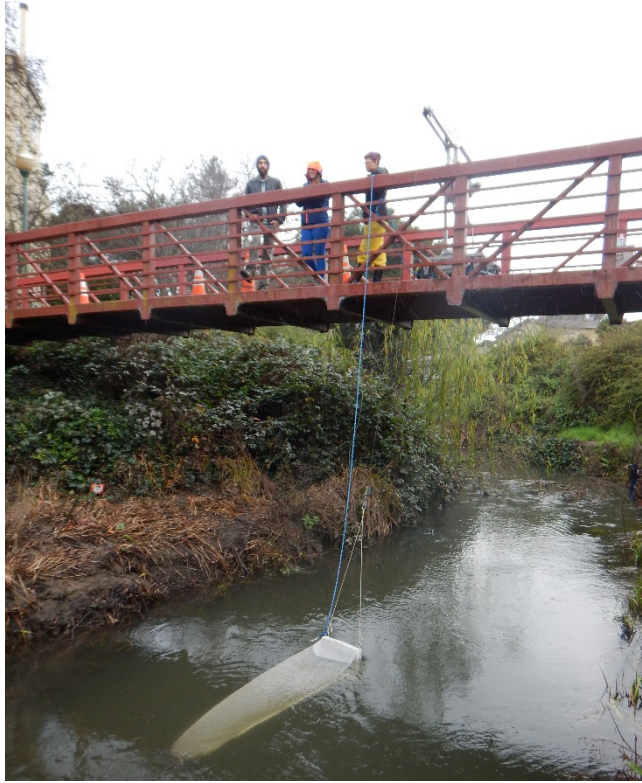
Figure 27. Rectangular Trawl deployed at San Mateo Creek
