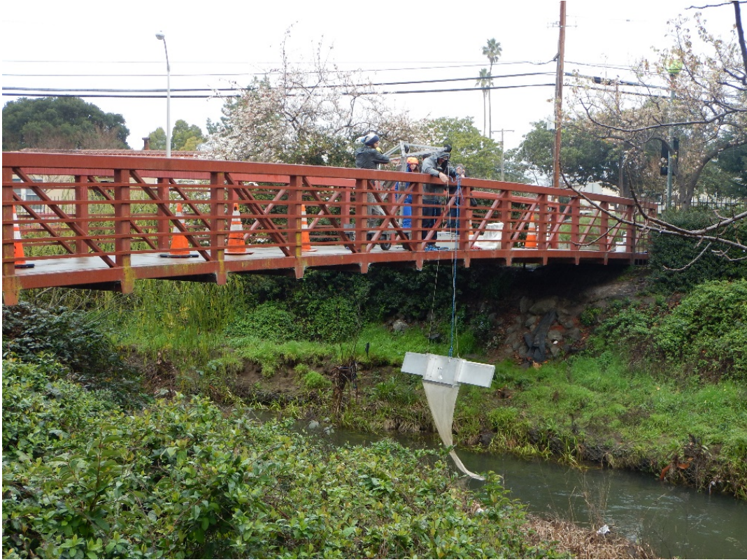
Figure 9. Manta Trawl bring deployed at San Mateo Creek
